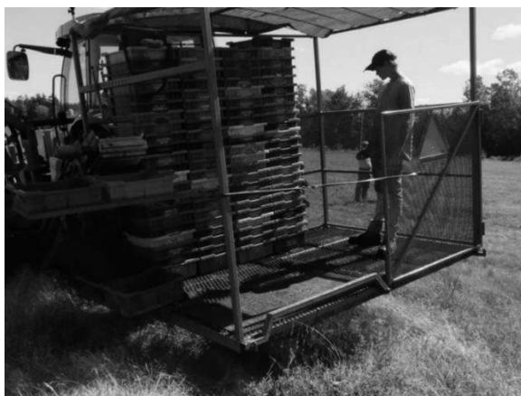
(b) Mechanical Harvester Illustrating Worker (at rear), and Small Box Handling System.
