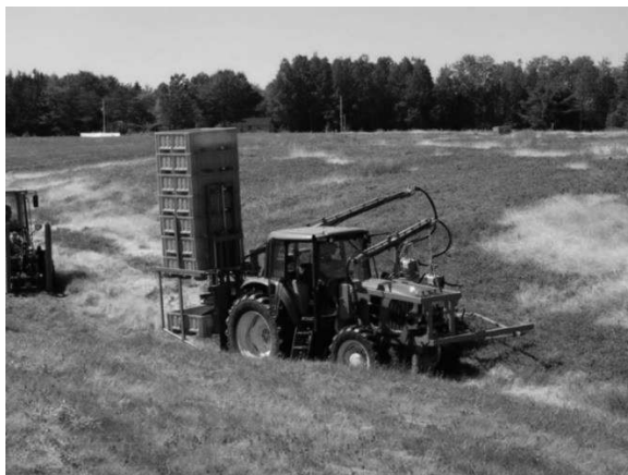
(a) Mechanical Harvester Illustrating Semi-automatic Bin Handling System.
